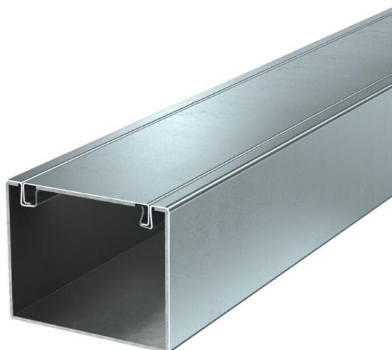
Metal installation duct with intumescent fire protection mesh for fireproof routing of cables. Classified as an installation duct EI30, EI60 and EI90 according to EN 13501-2, tested according to EN 1366-5. The duct prevents the fire spread for the classified period of time, offering protection against the effects of a cable fire.
