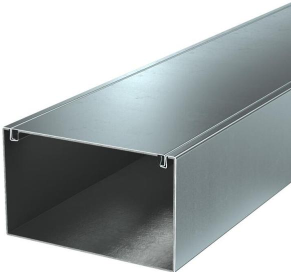
Metal installation duct with intumescent fire protection mesh for fireproof routing of cables. Classified as an installation duct EI30, EI60 and EI90 according to EN 13501-2, tested according to EN 1366-5. The duct prevents the fire spread for the classified period of time, offering protection against the effects of a cable fire.
