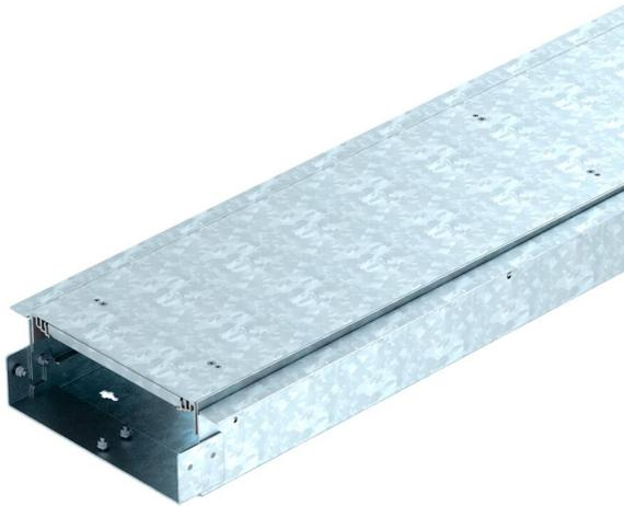
Ready-to-mount trunking unit for cable routing, consisting of a trunking base with two covers. The scope of delivery contains two lid butt seals and one connector. For height adjustment, six height adjustment units are required. Load capacity up to a maximum of 5 kN. The trunking unit can be supplemented with an adjustable floor covering contact profile for screed limitation in areas of door frames and in front of radiator niches.
