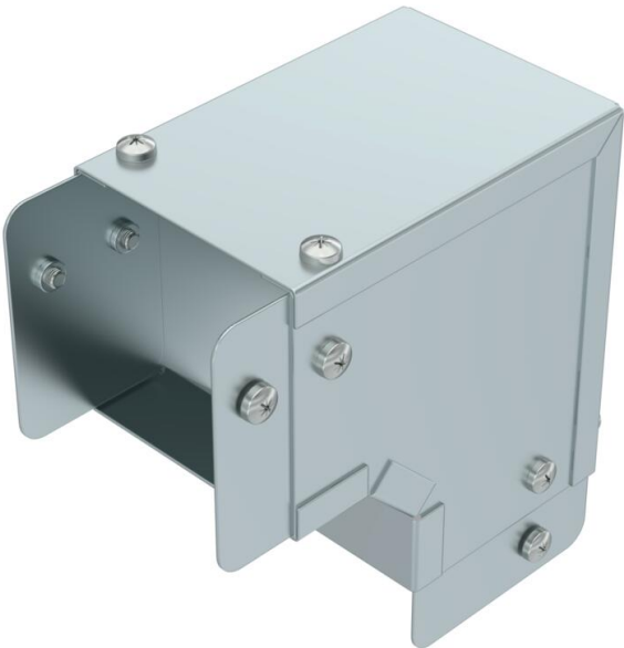
Single Compartment 90 Degree External Cover Bend, Pre-Galvanised Steel to suit Cable Trunking 75mm x 75mm
