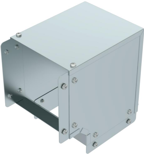
Single Compartment 90 Degree External Cover Bend, Pre-Galvanised Steel to suit Cable Trunking 150mm x 150mm
